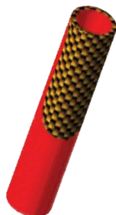
Pin-type fuel element of Gas Fast-cooled Reactor (GFR)
